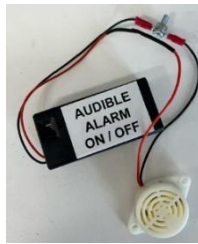
AA First Overflow Alarm
