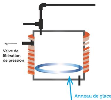
SYSTÈME DE REFOUILLISSEMENT ALIMENTÉ PAR UN RÉSERVOIR OUVERT
