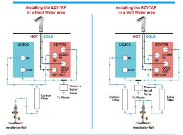
Installing the EZYTAP in a Hard Water area
