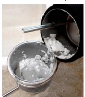
A hot tank can scale up in a relatively short time – depending on the water hardness, how hot the temperature and if there is high use.
