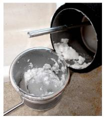
A hot tank can scale up in a relatively short time – depending on the water hardness, the hot temperature and with high use.
