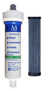
The NANOFilter consists of a nano fine carbon impregnated woven glass fibre material which is tightly folded to create a very large surface area. The Filter Candle fits into our standard Filter Housing. The very large surface area of the NANOFilter ensures an excellent flow rate and lack of blocking. It's fine weave and material properties are responsible for the outstanding Viral- and Pharma Ratings.
